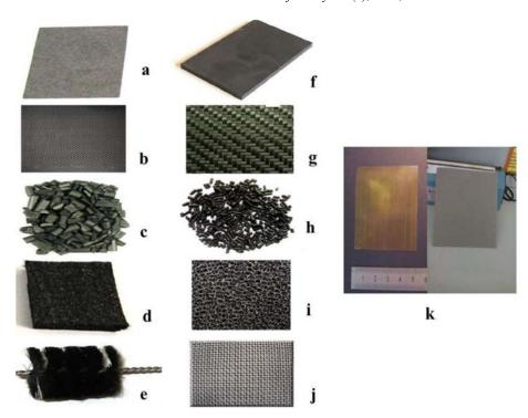
**Fig. 3.** Photographs of electrode catalyst or materials used for MEC: (a) carbon paper; (b) carbon cloth; (c) granular graphite; (d) carbon felt; (e) carbon brush; (f) graphite plate; (g) carbon mesh; (h) granular activated carbon; (i) reticulated vitrified carbon; (j) SS mesh; (k) electroformed Ni mesh.
