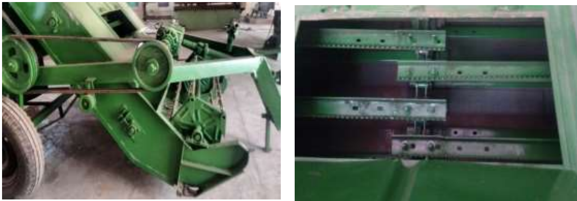
Fig. 2 Harvesting and densifying mechanism of collector-cum-chopper
