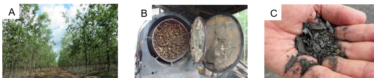
Figure 1. (A). Culture of A. mangium ; (B). Slow pyrolysis oven; (C) Biochar of A. mangium residues.
