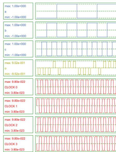
Fig. 11. Proposed three-input Majority Gate simulation results.
