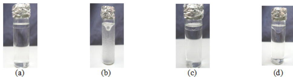
Figure 2. Illustration of the used apparatus for DSDME: (a) addition of the organic solvent to the aqueous sample solution, magnetic stirrer is off; (b) magnetic stirrer on, extraction occurring (T1); (c) addition of the acceptor phase droplet into the organic solvent, stirrer off; (d) magnetic stirrer on, back extraction occurs (T2) after the back extraction, droplet is withdrawn with the microsyringe.
