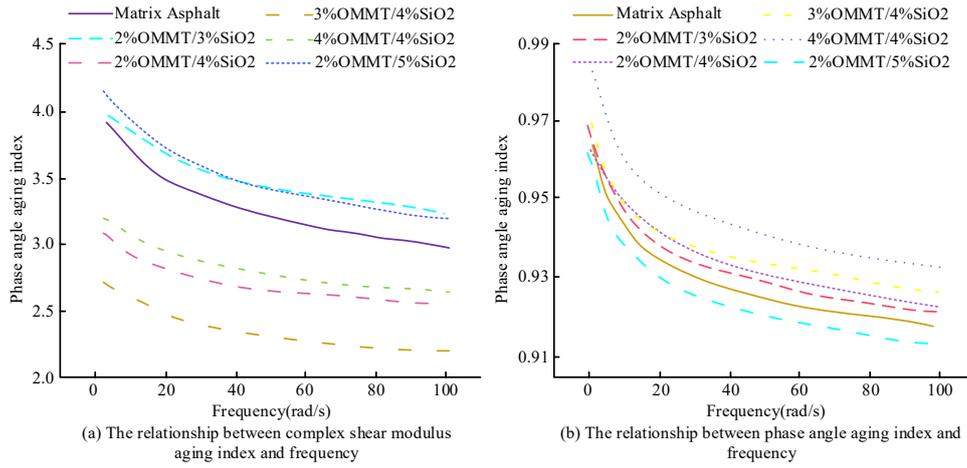
Figure 10. Relationship between the aging index and the scan frequency.
