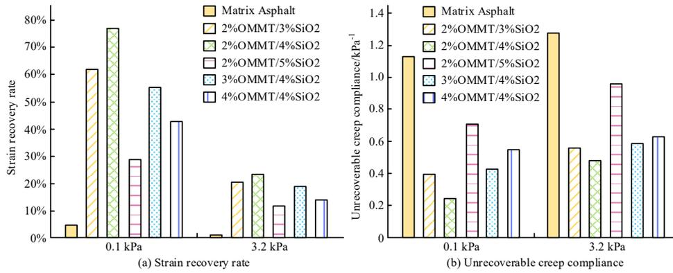
Figure 1. Results of multiple stress creep experiments.
