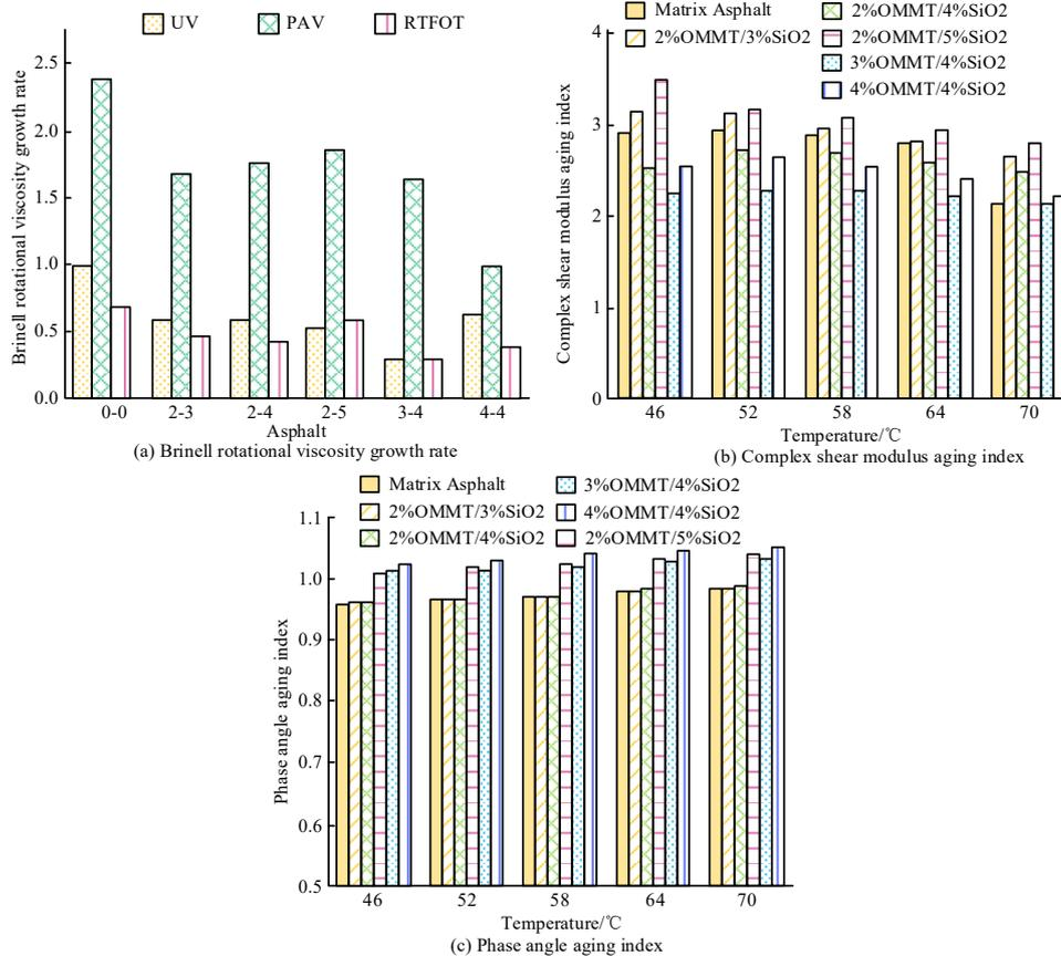
Figure 9. Growth rate of rotational viscosity and aging index after UV aging.
