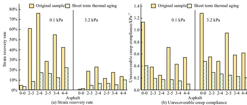
**Figure 4.** High temperature performance with short-term thermal aging.
