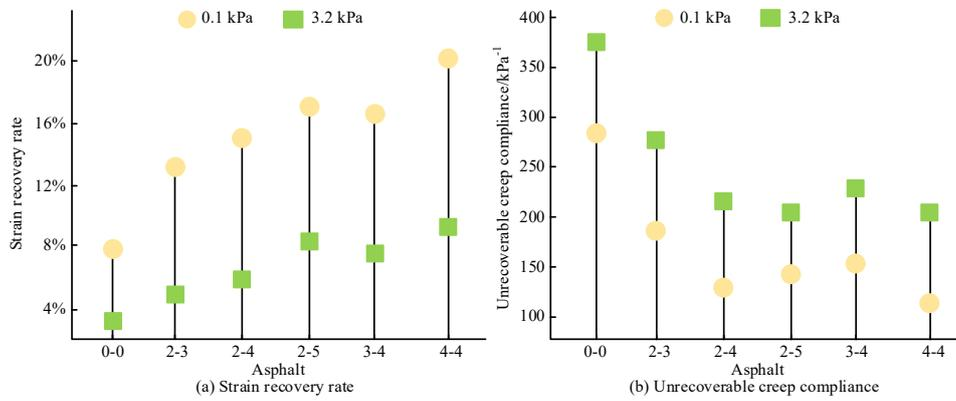
Figure 11. Results of multiple stress creep recovery experiments of UV-aged modified bitumen.
