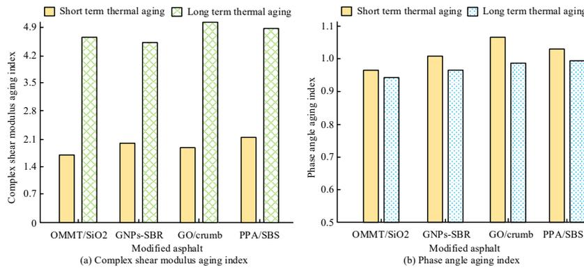
Figure 8. Aging index of different modified asphalt after thermal aging.
