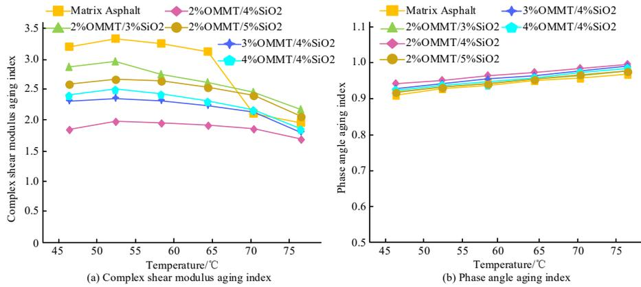
**Figure 3.** Results of the short-term thermal aging experiments.
