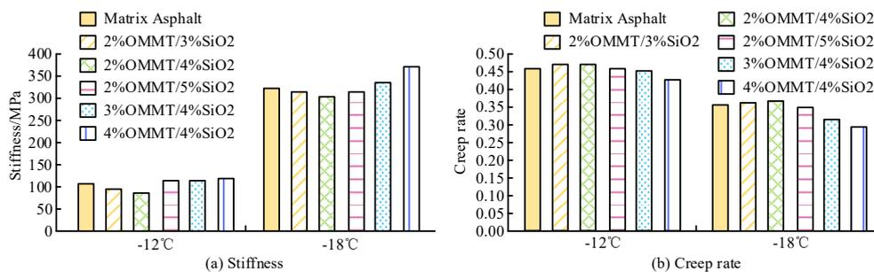
Figure 2. Results of the low-temperature bending beam rheology experiments.
