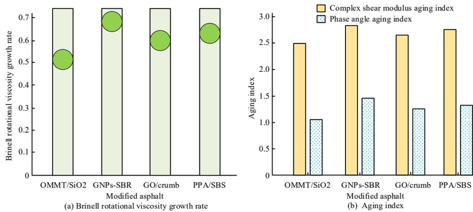
Figure 12. Growth rate and UV aging index of different modified asphalt.
