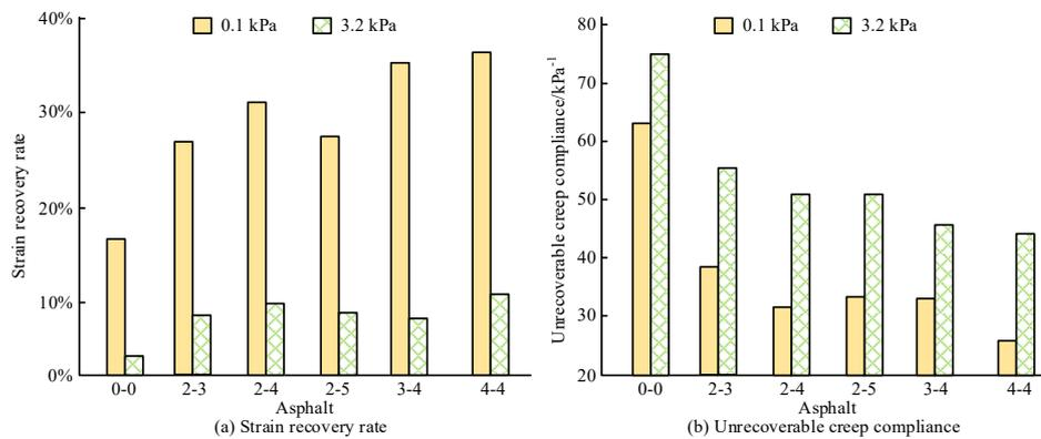
Figure 7. High temperature performance of modified asphalt with long-term thermal aging. Note: The x-y on the horizontal axis represents modified asphalt containing x% OMMT and y% silica.
