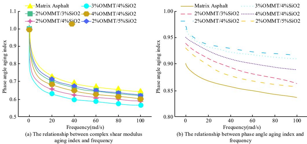
Figure 6. Relationship between the aging index and the scan frequency.
