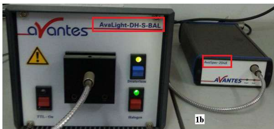
Supplementary Fig. 1b: Diffusive reflectance utilized to inspect the PMMA/TiO 2 films
