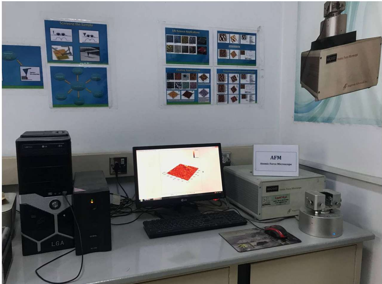
Supplementary Fig. 2: AFM (AA2000) to illustrate the surface roughness of PMMA/TiO 2 thin films
