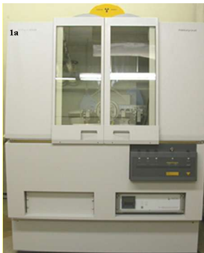
Supplementary Fig. 1a: XRD device utilized to inspect the structure of the nanocomposite films PMMA/TiO 2 , the diffraction angle ( 2\theta ) ranged from 10° to 80° to exhibit the film's structure crystalline or amorphous.
