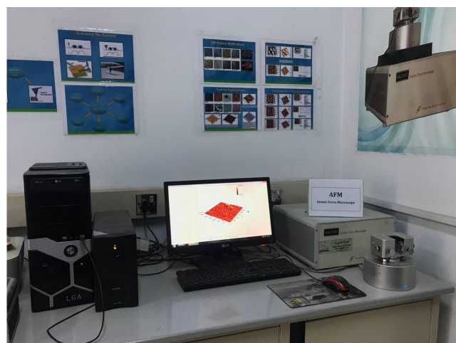
Supplementary figure 2. AFM (AA2000) to illustrate the surface roughness of PMMA/TiO 2 thin films.
