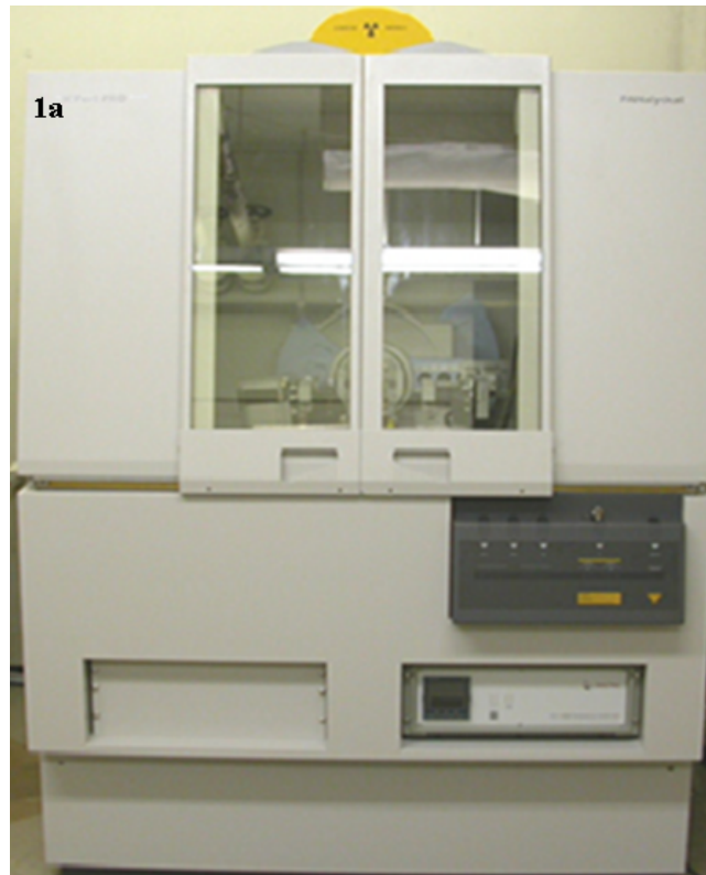
Supplementary figure 1. (a): XRD device utilized to inspect the structure of the nanocomposite films PMMA/TiO 2 , the diffraction angle ( 2\theta ) ranged from 10° to 80° to exhibit the film's structure crystalline or amorphous. (b) Diffusive reflectance utilized to inspect the PMMA/TiO 2 films.
