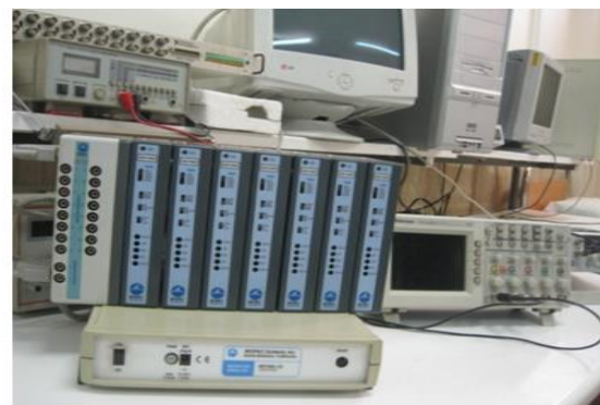
Fig. 3. The Biopack MP150 Device with its Modules and its connected amplifier modules is used for recording EOG signals.
