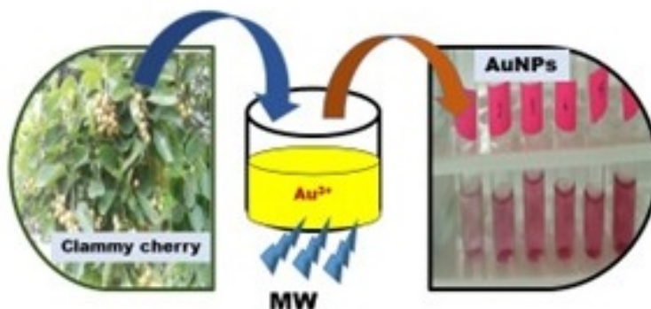
Figure 1. Pictorial illustration of MW-assisted synthesis of AuNPs using clammy cherry extract.
