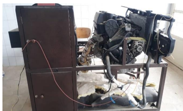
Figure 1. Photo of actual experimental setup (Engine for Peugeot-405 XU7)
