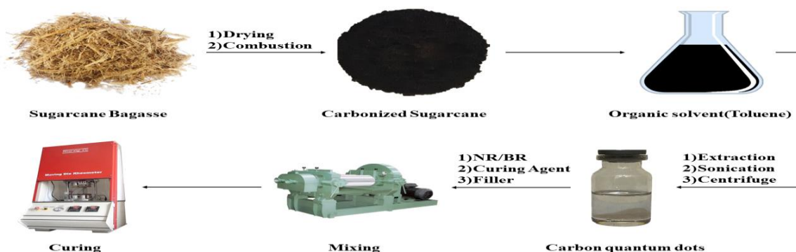
Scheme 1. Illustration of the manufacturing process of NR/BR nanocomposites
