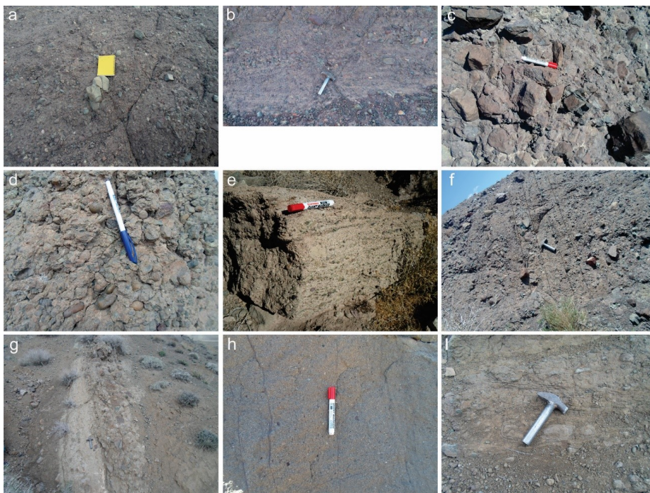
Figure 4. Selected outcrop views of conglomerate and sandstone lithofacies from the Kerman Formation; (a) Angular pebbles in poorly-sorted matrix in matrix-supported massive conglomerate (Gmm); (b) Normal grading in matrix-supported conglomerate (Gmg); (c) Angular pebbles in clast-supported massive conglomerate (Gcm); (d) Well-rounded pebbles in clast-supported massive conglomerate (Gcm); (e) and (f) Horizontal lamination in clast-supported, crudely bedded conglomerate (Gh); (g) Horizontal bedded, coarse to fine-grained sandstone (Sh); (h) Massive, coarse to fine-grained sandstone (Sm); (i) Faint lamination in massive, coarse to fine-grained sandstone
