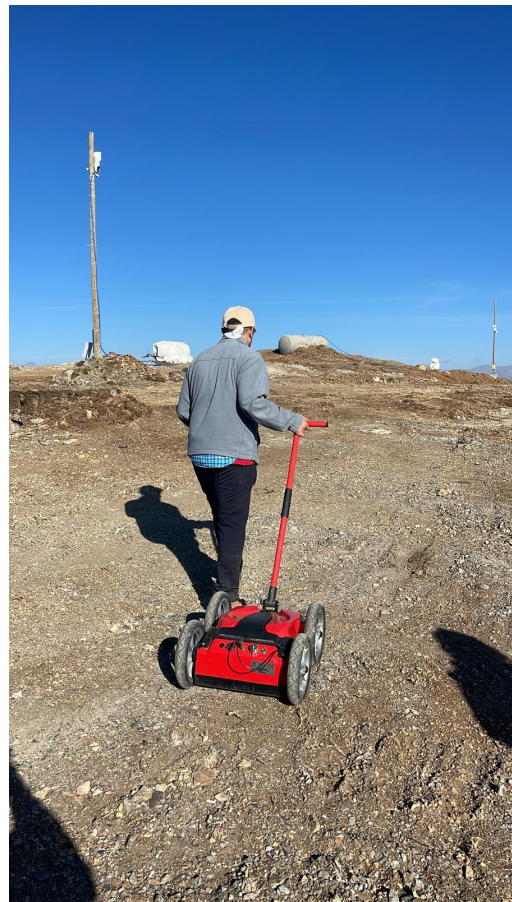
Figure 1. Measurement with Cobra GPR
