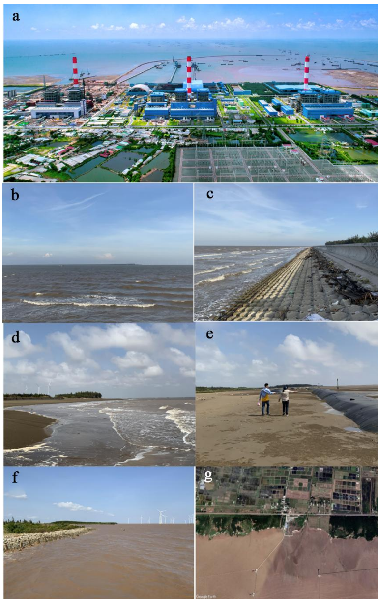
Figure 21. a) Thermal power station Duyen Hai 1 . b) the sand dune has connected to the mainland; c) the engineering works at Thua Duc beach; d) the beach at Ham Luong mouth with the engineering works; e) The Co Chien mouth used geotube to prevent erosion; f) an actual photo of the shoreline undulating (photo by the Bui Minh Quan), g) a Google Earth photo showing the shoreline undulating (photo by Google Earth)
