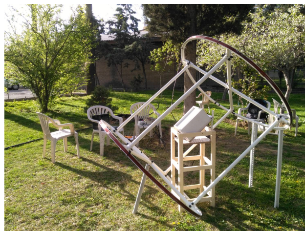
Figure 3. The experimental setup of the spin echo enhanced proton precession magnetometer.
