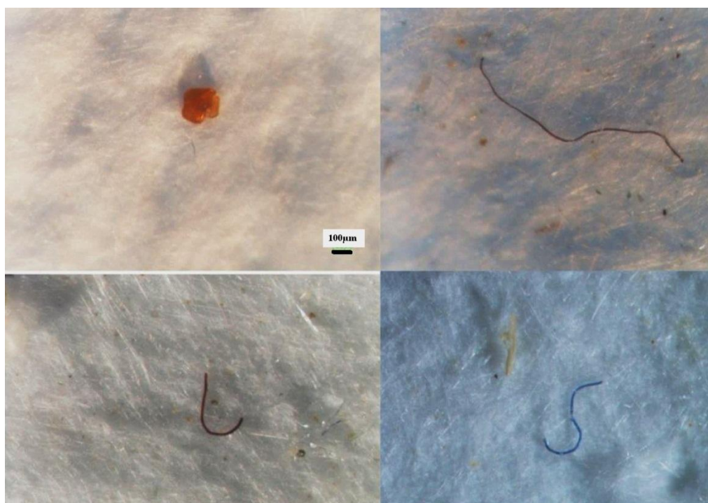
Figure 2. Representative optical micrographs of the collected microplastic
