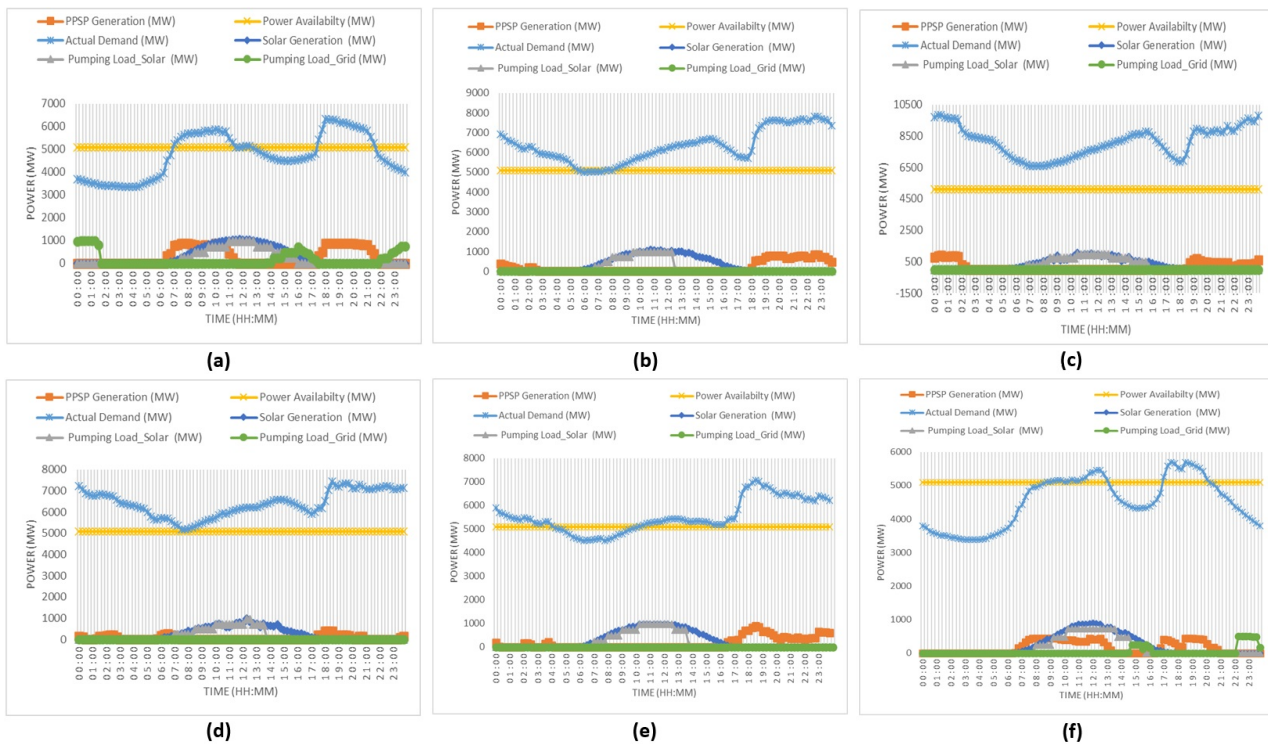
Figure 11. Actual load demand profile and hypothetical PPSP pumping using solar power and generation operation on (a) 6th February; (b) 26th April; (c) 8th June; (d) 24th August; (e) 4th October; (f) 30th December in the year 2023
