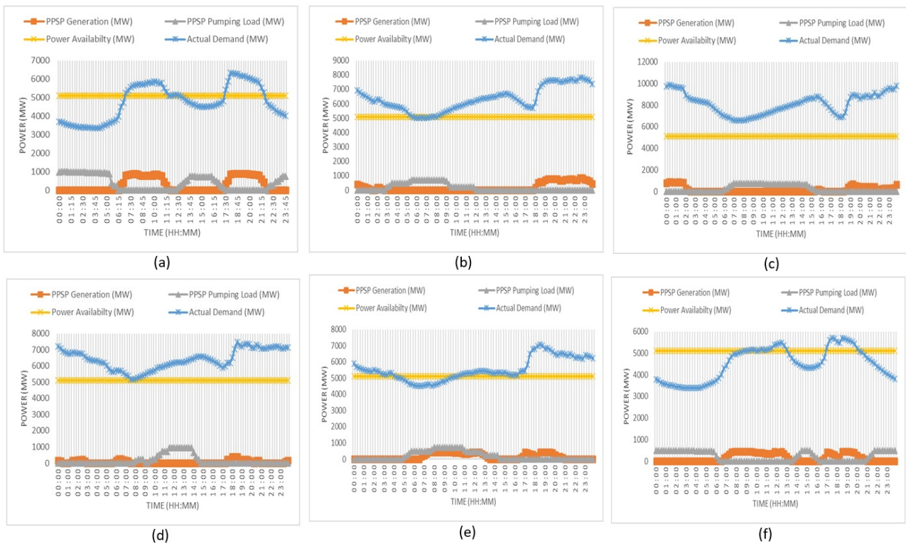
Figure 7. Actual load demand profile and actual PPSP pumping using grid power and generation operation on (a) 6 th February; (b) 6 th Feb., 26 th April, 8 th June, 24 th Aug., 4 th Oct., and 30 th Dec. of the year 2023.
