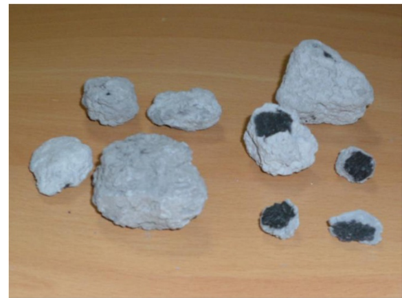
Figure 6 Fused bottom ash from the CFB furnace - small spherical sintered clay covering un-burnt lignite.
