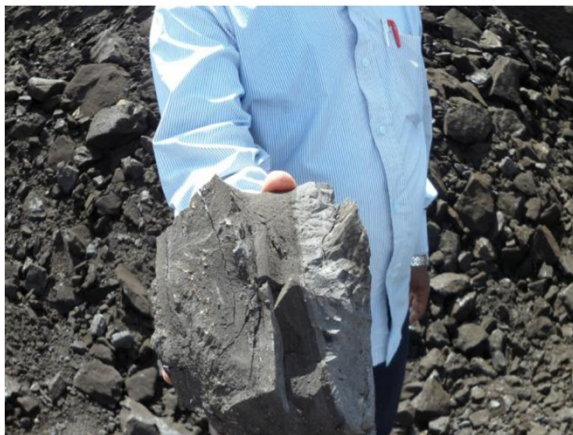
Figure 5 Photographs of mine lignite face - showing the mineral intrusions - halloysite clay (gray clay).
