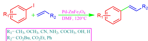
Scheme 21. Heck coupling reaction of Pd-Zn \text{Fe}_2\text{O}_4 .
