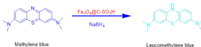
Scheme 2. Catalytic reduction of MB to LMB.
