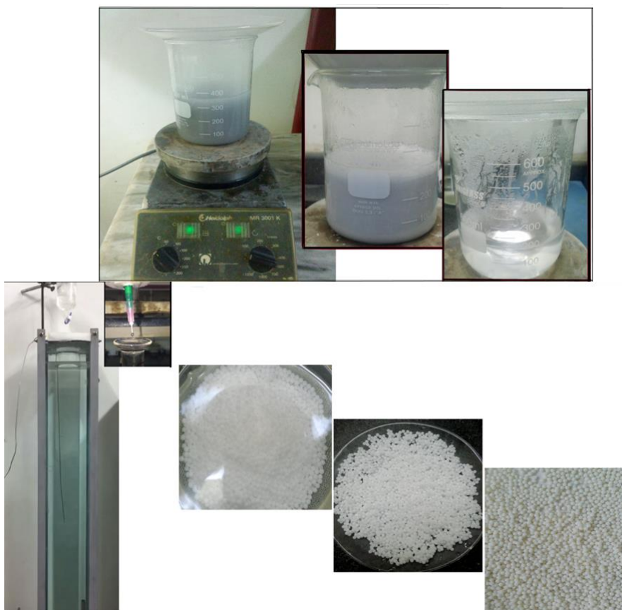
Figure 1. Several photographs of the spherical \gamma -alumina supports preparation steps
