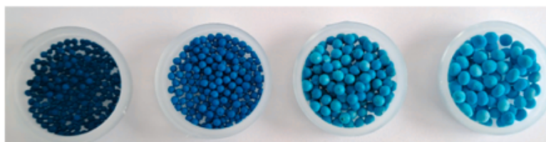
Figure 4. CS@HKUST-1[n(NH 2 ):n(Cu)] xerogels. From left to right: CS@HKUST- 1[2:1], [1:1], [1:2], and [1:3]. [Elsevier copyright 2024, with permission] [58].
