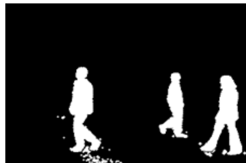
Figure 3. Foreground extraction of a moving person amidst background noise interference.
