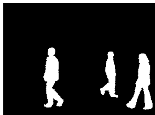
Figure 4. Refined separation of a moving person from the background following noise.
