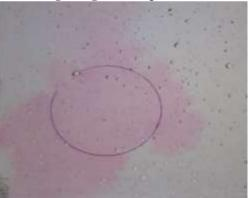
Figure 5 - Experiment on the concrete surface color of the sample with 2.5% titanium dioxide after 24 hours. Comparison of Figure 4 and 5 shows that self - cleaning properties were significantly affected by Nano TiO2.
