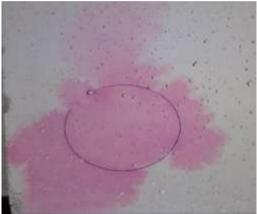
Figure 4 - Experiment on the concrete surface color of the sample with 2.5% titanium dioxide at the beginning of the experiment.
