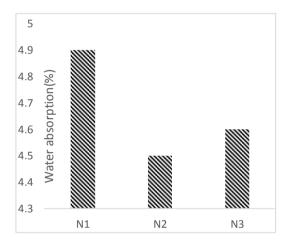
Figure 2- Comparsion of water absorption test as a result of adding of TiO<sub>2</sub> and Nano-silica in concrete
