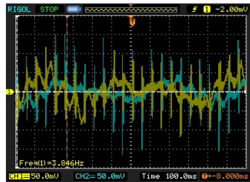
Figure 15. Experimental results of two stator phases voltage A and B at 3.1 m/s for (50m V/div, 100 ms/div).
