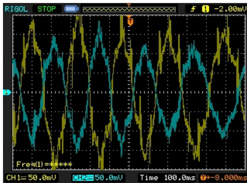
Figure 12. Experimental results of two stator coils voltage at 6 m/s for (50 mV/div, 100 ms/div).
