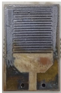
Fig. 1. a) The employed CO gas sensor. b) Changes in the sensor resistance as a function of the applied gas concentration to the sensor [۷۵].
