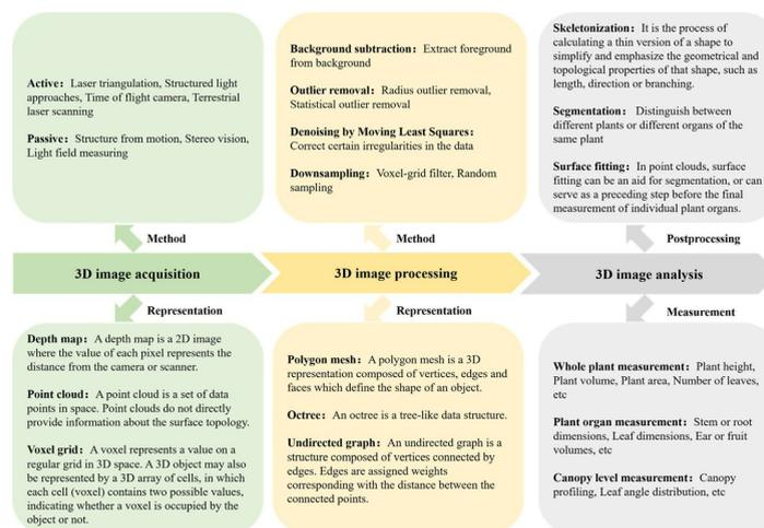
Fig. 2. The pipeline of 3D plant phenotyping.
