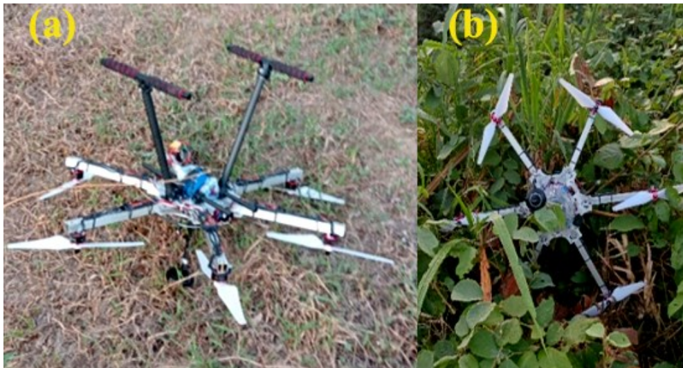
Fig. 6. A hexacopter testing using PID default (a) flip-over and (b) fell down in the bushes.
