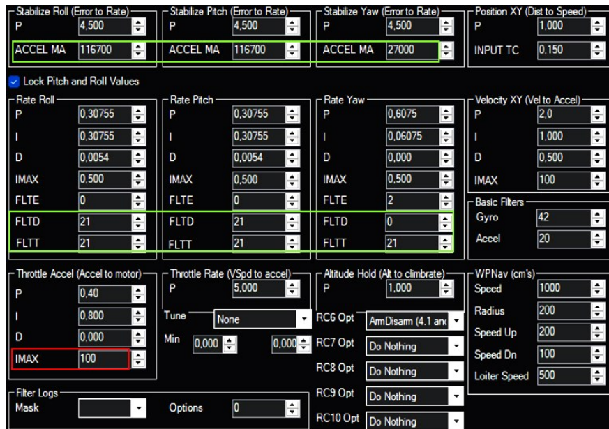
Fig. 9. A new PID tuning for DIY hexacopter with loads of 942 grams.
