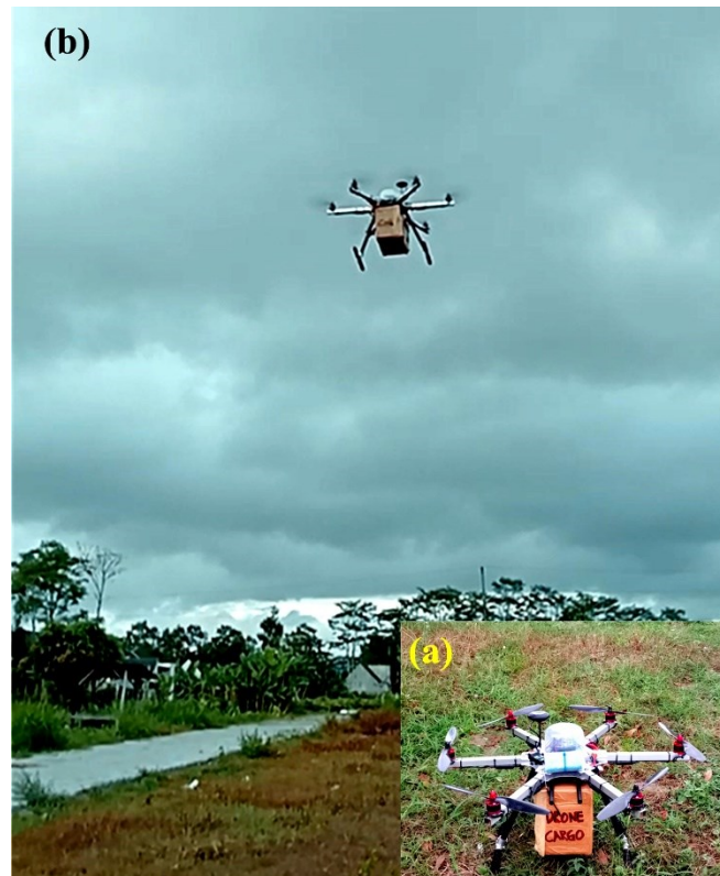
Fig. 10. Hexacopter testing using 10-inch propellers for drones with an additional load of 942 grams (a) in the takeoff position and (b) moving up to the first waypoint. All images in this work are original.
