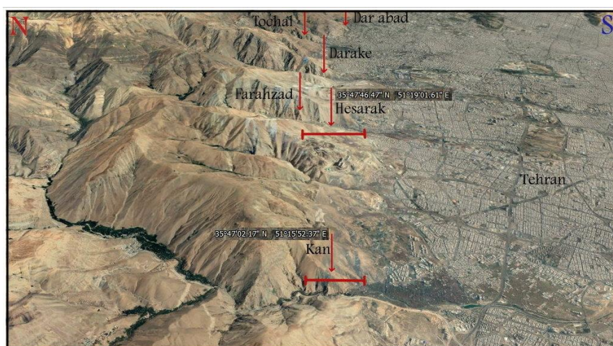
Fig 2. Signs in the shape of arrow are points along the fault that were surveyed during the study, but only the two areas of Kan and Hesarak, whose coordinates are written, were examined as typical sections.
