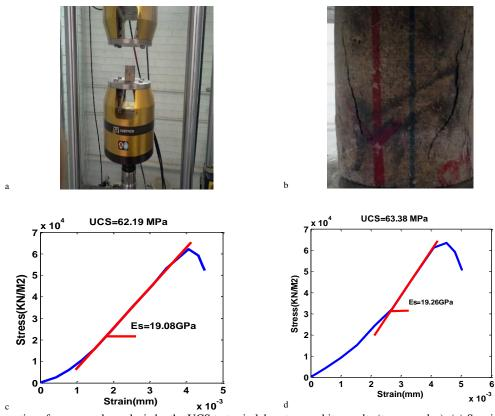
Fig 3. Schematics of core sample analysis by the UCS tester in laboratory and its results (two samples): (a) Specimen prior to the UCS test (b) Specimen after the UCS test (c) Stress and strain curve for core sample no. 2 (d) Stress-strain curve for core sample no.
