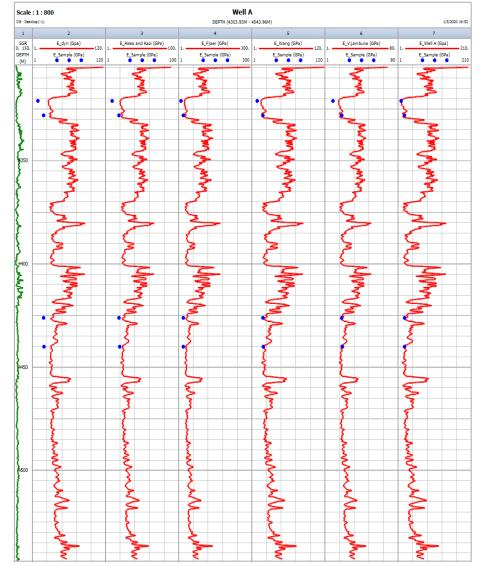
Fig 5. The Es estimation curves (red color lines) through utilizing empirical equations (Equations 2-6) and real Young's modulus data of the core specimens (blue points).
