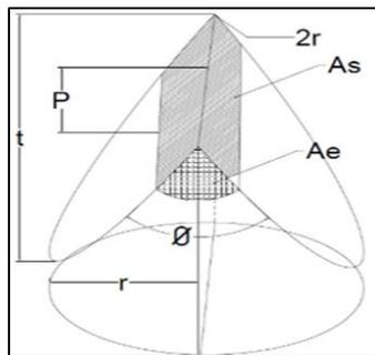
Fig 3. The geometry of the roller cutter bit.  $p$  is the vertical force acting on the rock to the penetration depth,  $\phi$  is the edge angle for a bit, and  $r$  is the cutter diameter.
