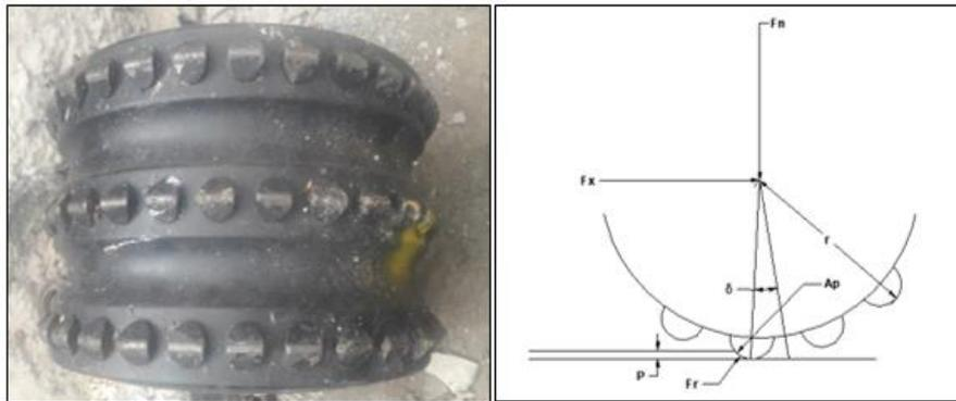
Fig 2. Reamer roller cutter.
