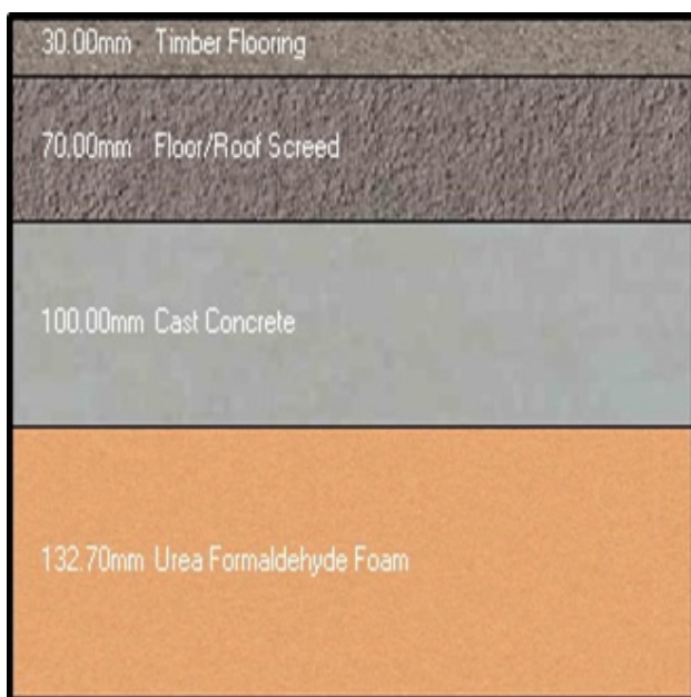
Figure 10. Schematic figure of the floor.
