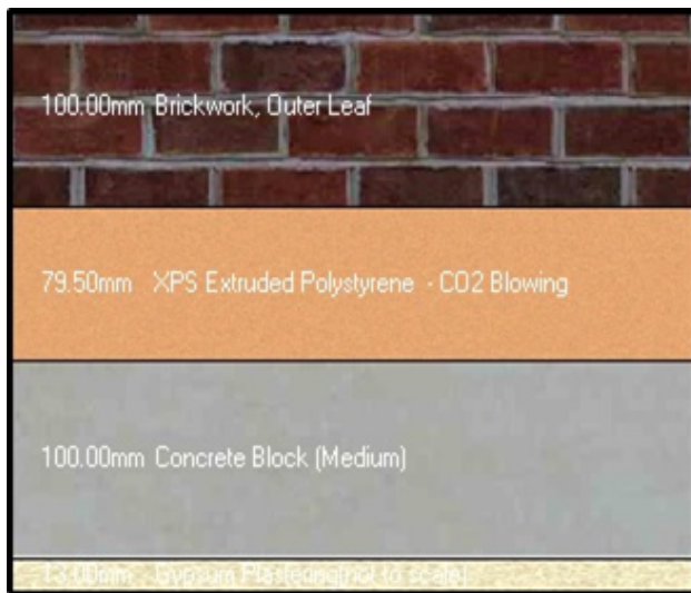
Figure 8. The schematic diagram of the external wall.
