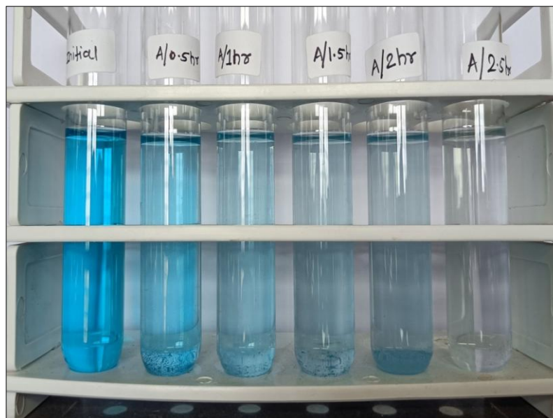
Figure 12. Photocatalytic degradation condition of turquoise blue G dye was assessed using 7% Cu:ZnO/TiO 2 after every 0.5 hour
